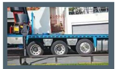
Fitting everything needed on the truck was a challenge. Note the 'extra long' load frame and tank lifter built into the top of the tail board. Foot pads are tucked neatly behind the drop guards
