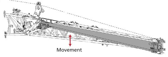
In this transport configuration the tip section is leveraged by its own weight. This combined with the road conditions can place additional pressure on different components. In this event, the movement led to a component failing. The tip section then opened on the transporter into the live traffic lane with the potential to cause serious harm.
