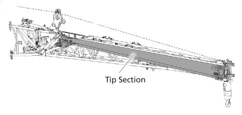
The load was secured to the transporter by a single strap at the front and another single stap at the rear of the Jib. The tip section was secured using only the manufacturers pining mechanism and components.
