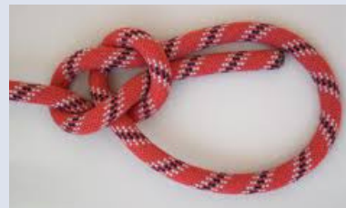
Bowline: a common tagline knot
