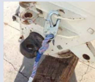
Clip termination on a tagline
