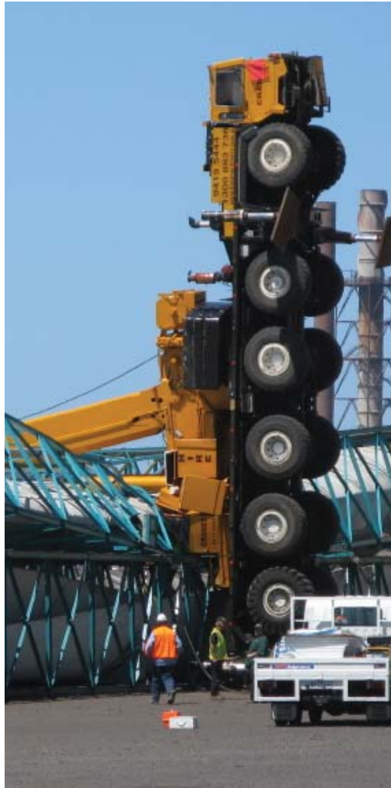
Port Kembla, south of Sydney and a 150 tonne crane goes end up. Emergency service workers braved a constant shower of diesel fuel to rescue the trapped operator, who escaped with a broken leg.
